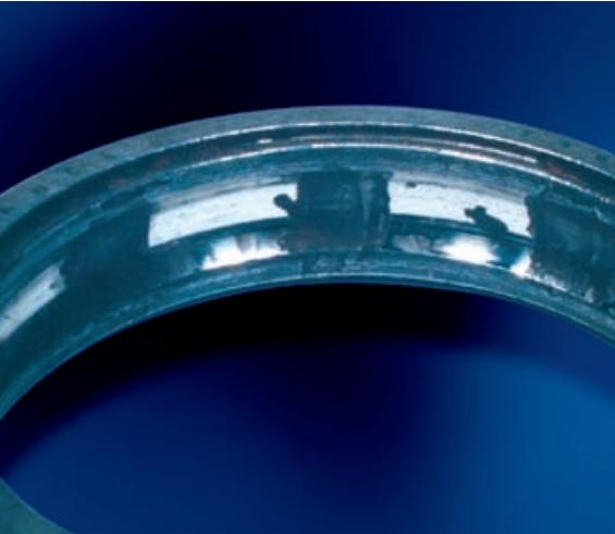
Corrosion when operating (liquid ingress)
