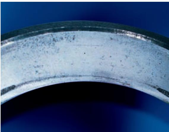
Cone spalling due to taper of the shaft or housing
