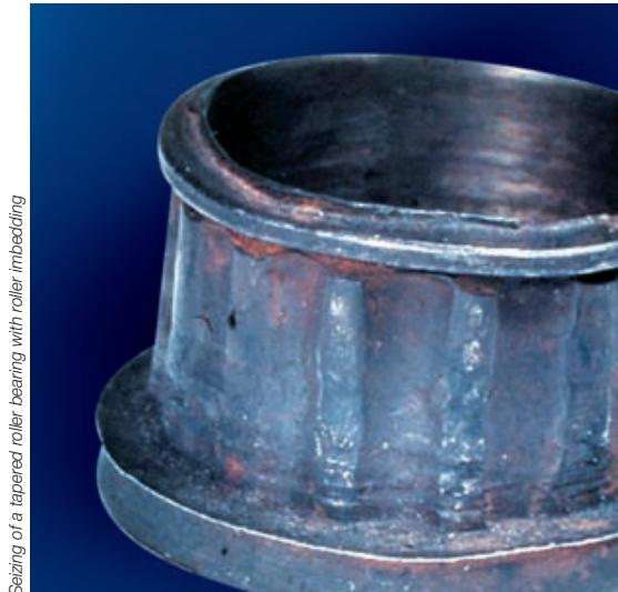
Seizing of a tapered roller bearing with roller imbedding
