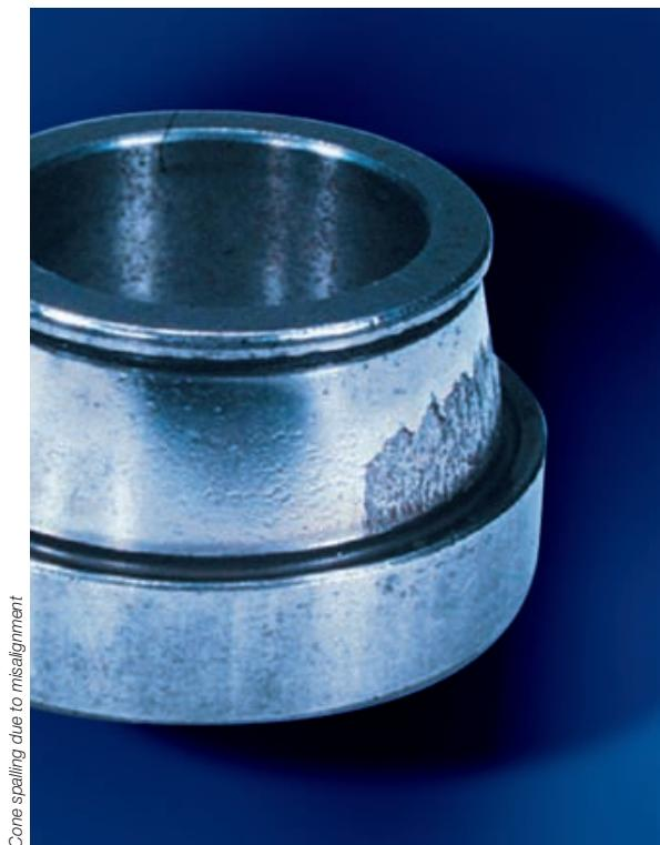
Cone spalling due to misalignment
