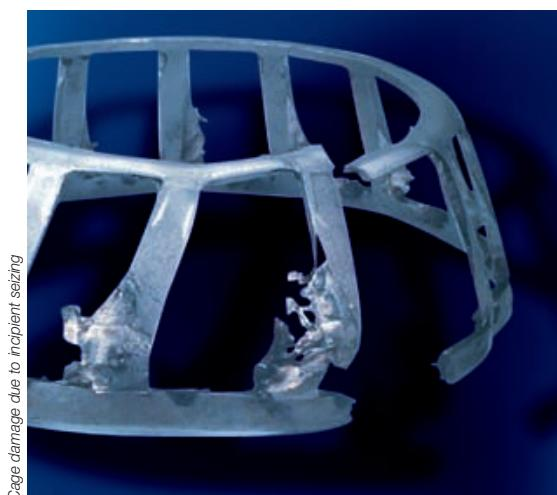
Cage damage due to incipient seizing
