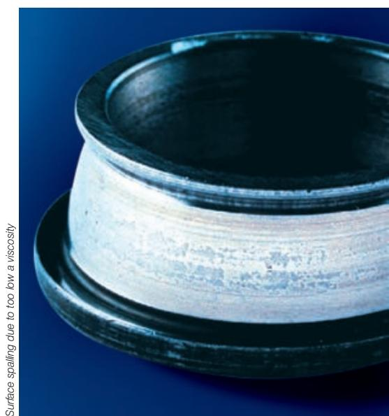
Surface spalling due to too low a viscosity
