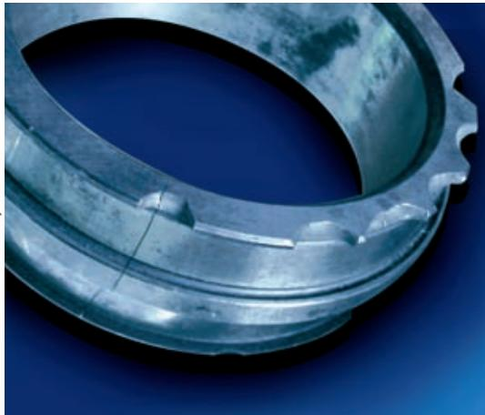
Fracture due to force-fit assembly
