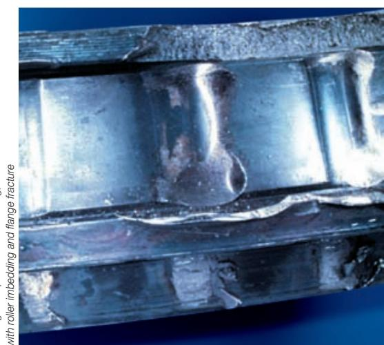
Seizing of a spherical roller bearing, with roller imbedding and flange fracture
