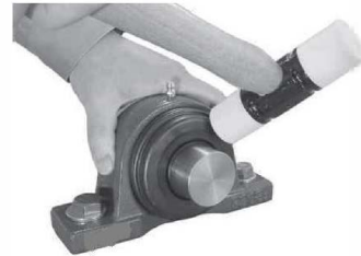
Fig.8.12 Installing steel plate covers
