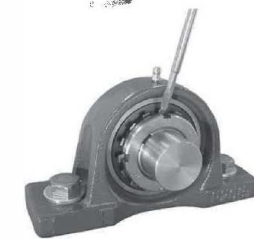
Fig.8.8 Bending claw of washer (Locking locknut)
