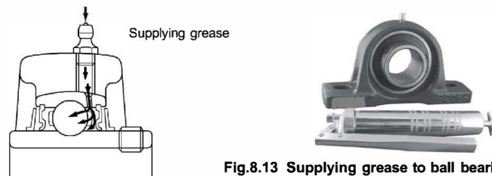
Fig.8.13 Supplying grease to ball bearing units
