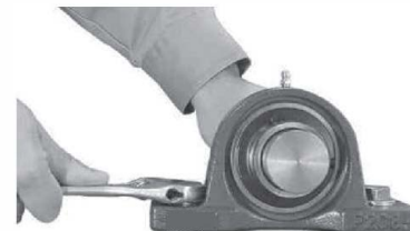
Fig.8.4 Installation of setscrew units
