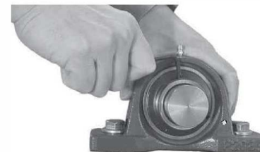
Fig 8.5 Tightening of set screws
