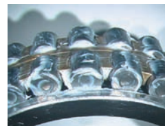
Photo. 6.2 Filling grease into cylindrical roller bearing
