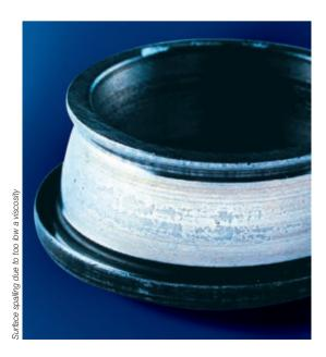
This failure is characterized by the appearance of grayish marks of varying extent on the raceway surfaces and in the load zone. A microscopic examination will show that the metal is only superficially affected.
