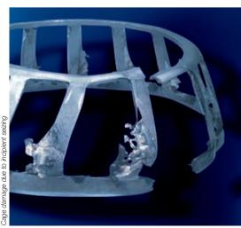
High speeds can also generate seizing when the bearing load is light. Rolling elements may not rotate instantaneously, either because of their inertia, or because of a rotational slow down caused by the lubricant. Friction generates a temperature rise and the resulting expansion causes seizing between rolling elements and raceways.
