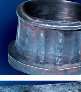
and flange fracture Seizing of a spherical roller bearing, nbeddina
