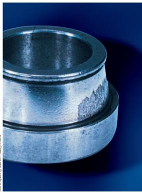
Cone spalling due to misalignment
