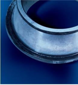
Damage to the flange due to excess preload
