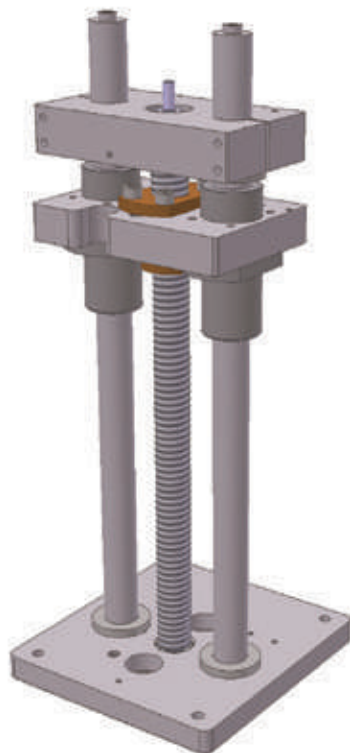
Figure 8.7 ___ AXLX_T Ball bushing table - Special Special design with trapezoidal screw drive
